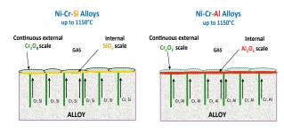
**Ni-Cr-Si** materials build protective oxide scales through the synergistic effect of the elements chromium and silicon. The dominating chromium oxide scale  $(Cr_2O_3)$  reliably protects the material up to temperatures of 1150°C against high temperature corrosion attack. Silicon supports the growth of the chromium oxide scale.
