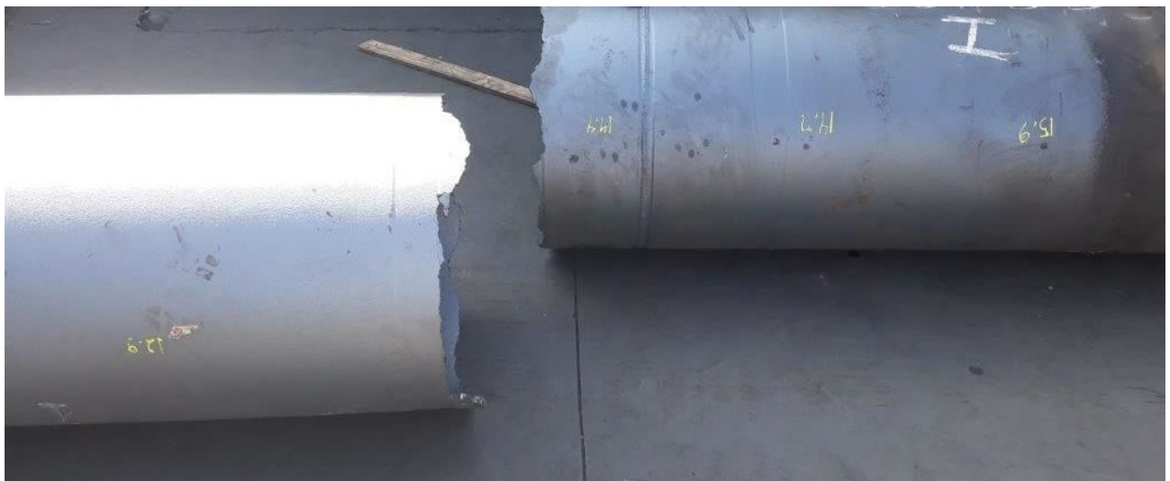
Fractured rotary kiln for investigation of failure Result of examination: Local overheating
